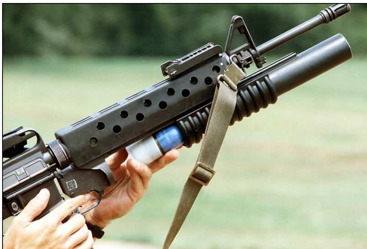
Loading an M203 attached on an M16A1 rifle. The grenade's blue tip and white body shell indicate it is a practice round.
