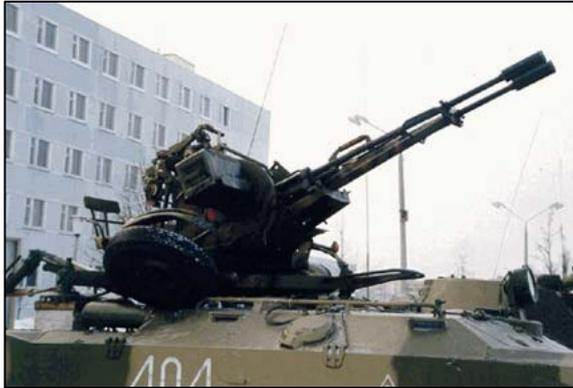
From all of the crew members only two of them take part in firing placed in their combat seats on the upper part of the mount. One of them operates the ZAP-23 sight by inserting manually approximate target data to turn collimator sight, insert altitude and overtake angles. The other member is a gunner. He is holding collimator sight's cross on the moving target.
