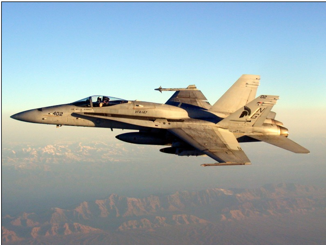
F/A-18C/D Hornet , side number 402 VFA-147 of the Argonauts, embarked on the USS John C Stennis in the Arabian Sea.
